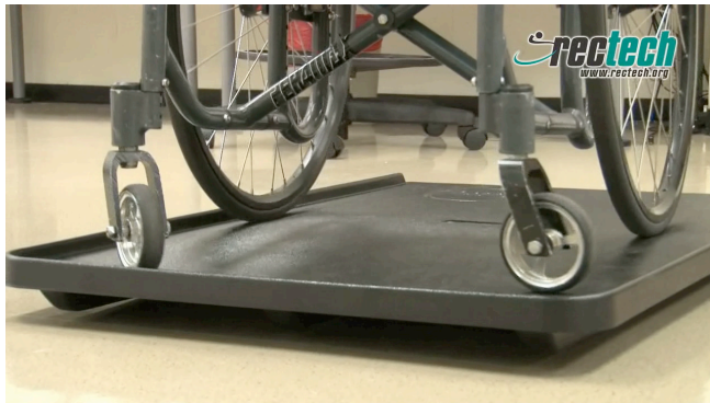
Figure 1. A large platform which sits on top of the Wii Balance Board as an example of an adaptation to allow wheelchair users to play games which require use of the balance board.
